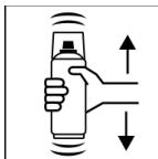
After activating, shake can again thoroughly for 2 minutes, again from when the mixing balls are heard.
